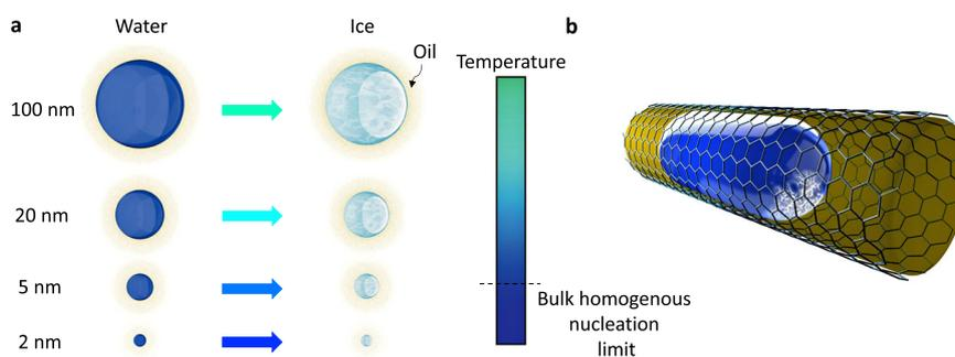
**Fig. 1** Freezing of water nanodroplets. **a** The length dependence of water–ice transformation in a heterogeneous mode. For 2 nm water droplets, heterogeneous nucleation could break the limit of bulk homogeneous nucleation. **b** Schematic of a nanodroplet formed in confined geometry and surrounded by an oil environment where ice nucleation occurs at the soft oil–water interface. The ice nucleation changes the local curvature of the oil–water interface.
