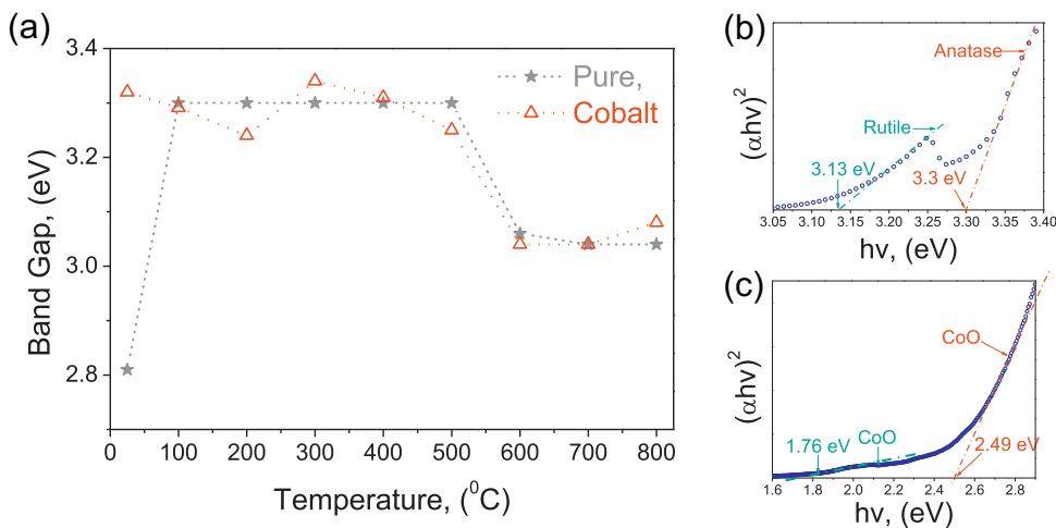
**Fig. 2.** Bandgap results of the (a) as synthesized and heat treated  $\text{TiO}_2$  with Co additions. The Figures in (b–c) are the bandgap results for (b) pure  $\text{TiO}_2$  heat treated at 500 °C and (c)  $\text{CoO}-\text{TiO}_2$  heat treated at 800 °C. Notice in (b and c) are shown more than one bandgap that is due to the presence of multiple phases typical of  $\text{TiO}_2$  and  $\text{CoO}$ .
