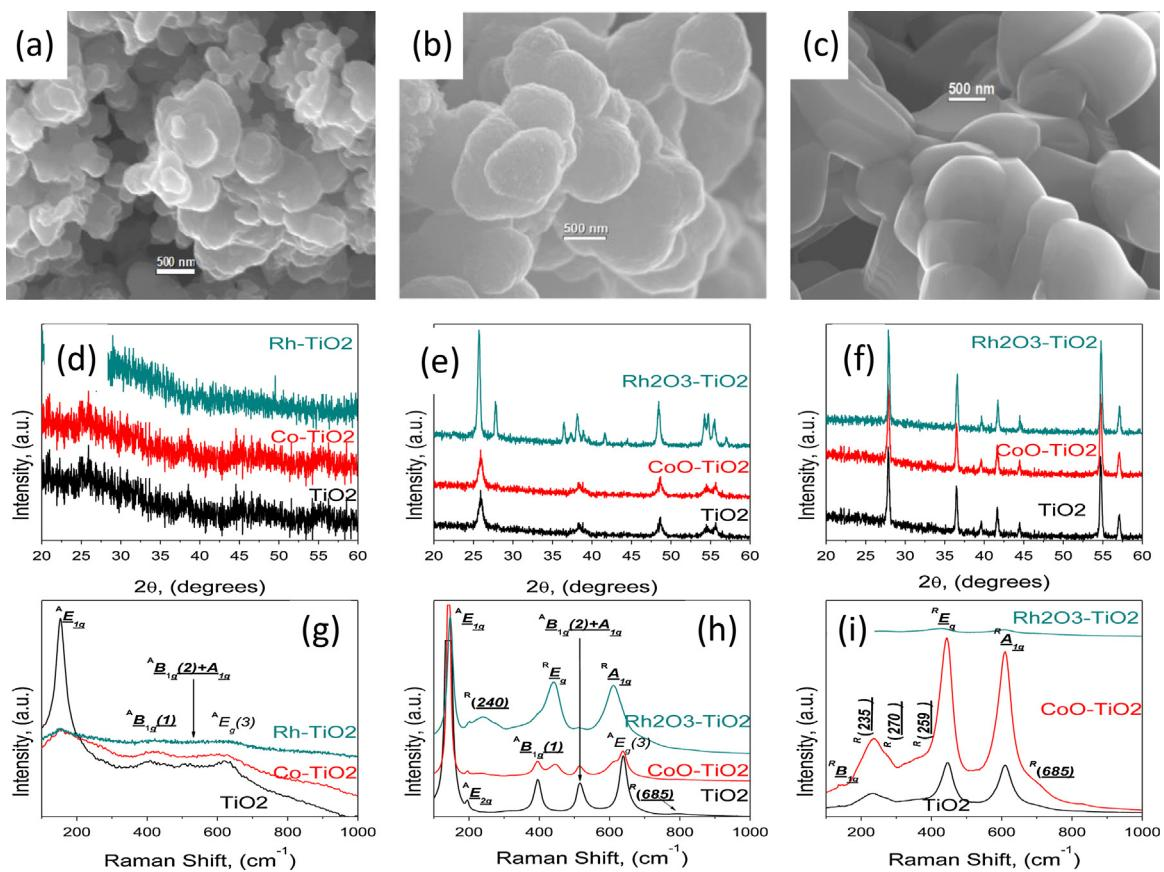
**Fig. 1.** Characterization of the as synthesized and heat treated samples by means of (a–c) SEM, (d–f) XRD and (g–i) Raman Spectroscopy. The results correspond to the samples in the following conditions: (a,d,g) As synthesized samples, (b,e,h) samples heat treated at 300 °C and (c,f,i) samples heat treated at 800 °C. Note: In the Raman spectrum the upper left letters (A or R) denote anatase or rutile respectively.
