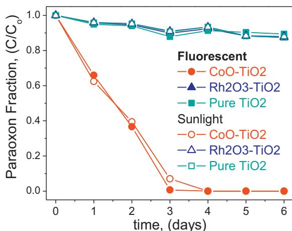
**Fig. 5.** Results of photocatalytic degradation of paraoxon using pure TiO<sub>2</sub>, CoO-TiO<sub>2</sub>, and Rh<sub>2</sub>O<sub>3</sub>-TiO<sub>2</sub> for duration between 1 and 6 days.
