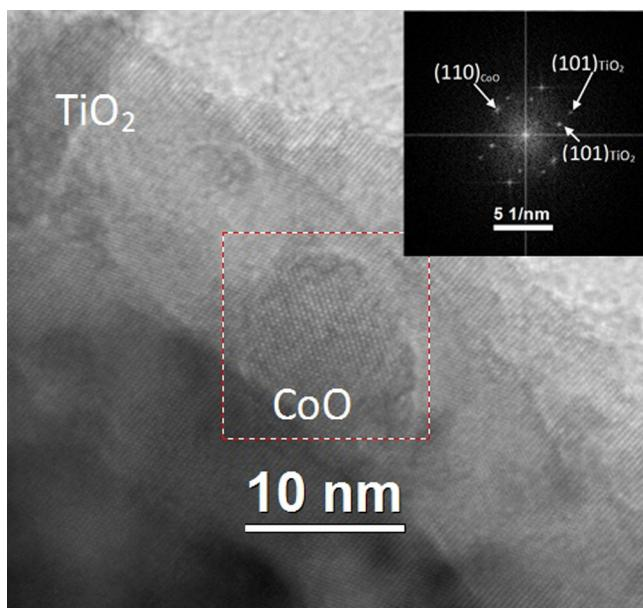
**Fig. 6.** The HRTEM of the  $\text{CoO}-\text{TiO}_2$  showing the “substrate” of  $\text{TiO}_2$  “decorated” by a particle of  $\text{CoO}$  (dotted square). The insets on the right upper corner shows the FFT of the dotted square region showing a dual pattern further confirming the presence of both phases ( $\text{CoO}$  and  $\text{TiO}_2$ ).
