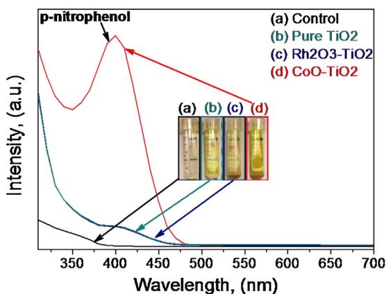
**Fig. 4.** Catalytic degradation of paraoxon using various catalyst and a control sample. The efficiency of the Co-TiO<sub>2</sub> is clearly evident when compared to the other tested samples, the experiment presented herein was carried for 1 day under sunlight conditions. Furthermore, the control sample do not show evidence of the degraded species.
