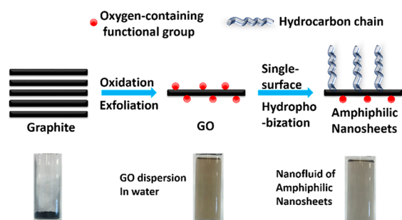
Scheme 1. Synthesis of Nanofluid Containing Graphene-Based Amphiphilic Janus Nanosheets
